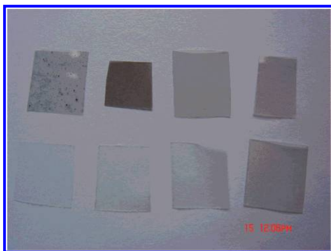
Figure 9. Photos of PS composite films containing different SWNT contents, prepared by a solution spin-casting method. The tube content in composite films in the first row decreases from left to right (0.12, 0.06, 0.045 wt %), and the first one is the unfunctionalized SWNT–PS composite film (0.10 wt %); the tube content in the second row decreases from right to left (0.022, 0.015, 0.011 wt %), and the last one is the blank PS film.
